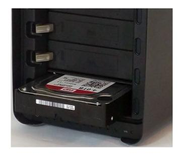
No tools are required for inserting hard drives, pull the locking thumb latch to the side and insert the hard drive. I will lock in place with in final position.
